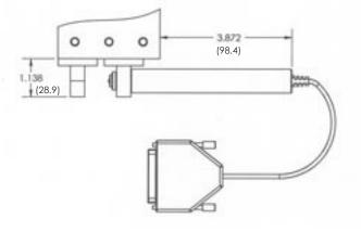
SIDE DRIVE 1" (25MM) MOTORIZED ACTUATOR (Dimensions shown with VB3/VR3, (VBM3/VRM3))
